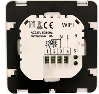
WiFi control: Please connect L and N to 220 voltage power, 5 and 6 to your gas boiler. 1 and 2 are for thermal actuators, please do not connect them to your gas boiler.
