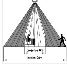
Height of installation: 2.2-6m Detection Distance: Max.20m
