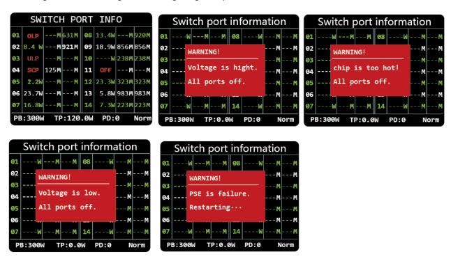
In addation, The third generation colorful LCD display add colorful logo display, upload and download speed of every port and ten interface setting functions base on the second generation LCD Display. The ten interface setting functions is include of Switch Mode, Band Width Warning, PD Type Setting, PSE Power Fine, PSE Port Priority, PSE Port Enable, Fan Control, Language, Factory Setting, Factory Setting.
