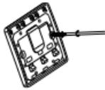
② Fix into expansion screw in the wall or 86 type switch box
