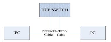
As shown in this figure, the version files are stored on the PC that is connected to the IPCs through the network.
