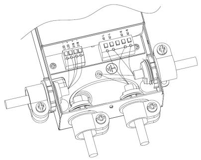
Remark: when you insert in or pull out the wires from the terminal blocks, please press and hold the terminal blocks until you finish the wire installation; the terminal blocks are suitable for AWG16-20 wires, and the skinned wires' length should be 6-7mm, the wires' skinned copper part should not be bare out of the terminals.
