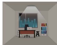
3. After elapse of hold time, the sensor dim to 20% brightness if no new motion detected.
