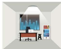
2. With insufficient ambient light, the sensor turns on the light and dim to 100% brightness when motion is detected.
